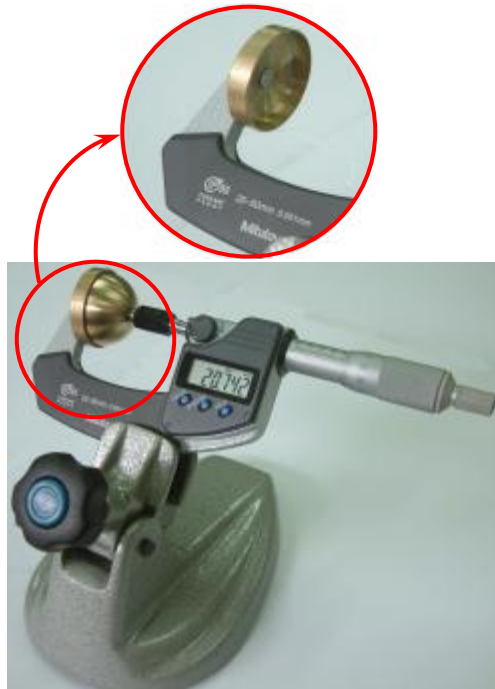
Figure A4: Measuring the plastic deformation using a micrometre.
