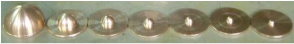
Figure A2: Hemisphere specimens with different radii.
