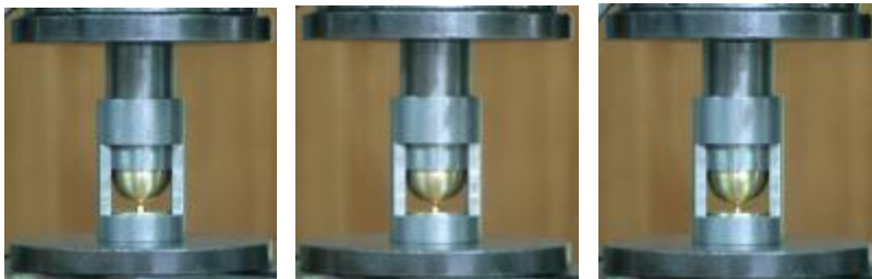
Figure A3: Hemispherical specimen couples.
