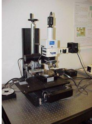
Figure B2: Interference microscope (Micromap) for measuring the topography of a real rough surface.
